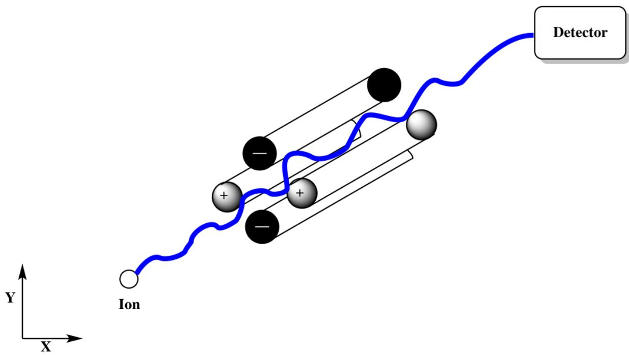
of the instrument resolution was low. Quadrupole design eliminated the use of magnetic fields altogether and replaced them with electric fields. Using these electric fields, ion trajectories are more stable and convenient for detection.
