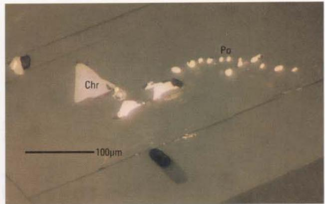
**Figure 5.** Photomicrograph showing symplectic chains of Ni-bearing pyrrhotite (Po) droplets in hornblende in basalt. Olivine and hornblende commonly enclose chromite (Chr) (sample 920814-11A). Scale bar corresponds to 100 μm.
