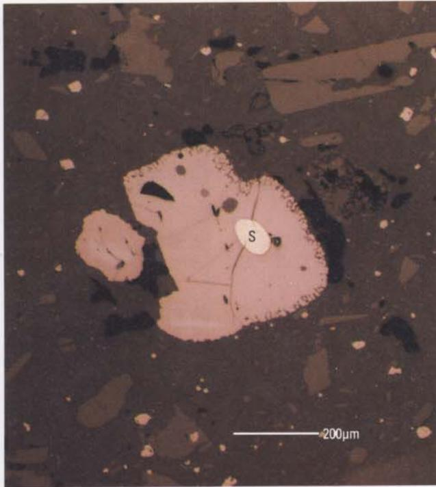
**Figure 3.** Photomicrograph of a rounded cubanite grain (S; 120 μm long) enclosed in ilmenite<sub>ss</sub> in dome andesite (sample 920814-10).
