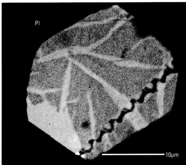
**Figure 15.** Back-scattered electron image of sulfide in 3-mm-long plagioclase (Pl) phenocryst (sample PP1-C-A).
