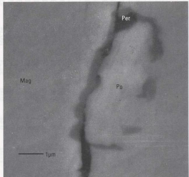
**Figure 10.** Back-scattered electron image of Ni-bearing pyrrhotite (Po) in magnetite<sub>ss</sub> (Mag). Dark phase between sulfide and oxides is perovskite (Per). Sample (CH1BE-W) is a dome andesite.
