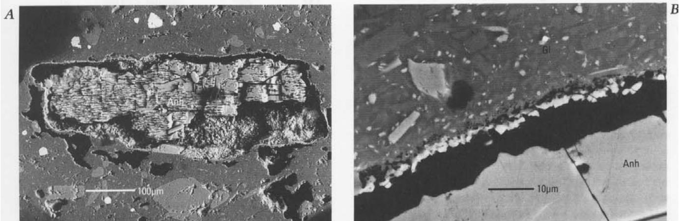
**Figure 2.** Back-scattered electron images of anhydrite (Anh) in dome andesite. *A*, The reaction rim, only 10 µm wide, is well exposed in the lower right because anhydrite was plucked out during the section preparation (sample CN1B-C). *B*, Boundary
