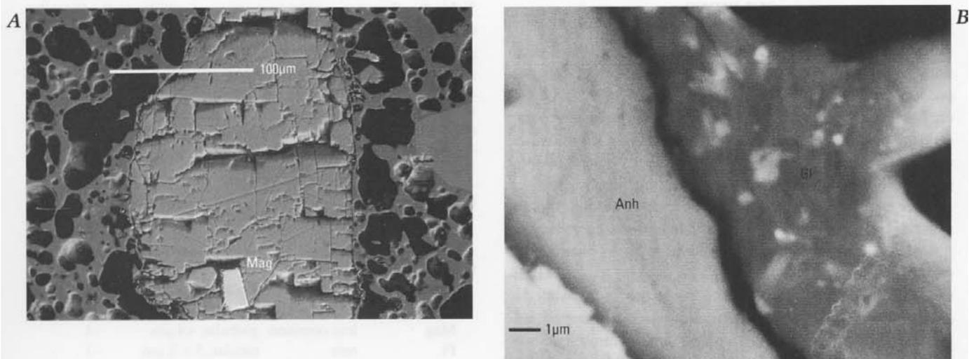
**Figure 1.** Back-scattered electron images of anhydrite in pumice. *A*, Anhydrite enclosing low-titanium magnetite (Mag) in banded pumice. *B*, Contact between anhydrite (Anh) and glass in white pumice. Note smooth boundary between the two phases. White specks in glass are microphenocrysts.
