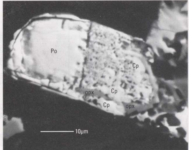
**Figure 9.** Reflected light photomicrograph of a symplectitic mixture of very fine grained magnetite, orthopyroxene (opx) and chalcopyrite (Cp) replacing Ni-bearing pyrrhotite (Po). Quantitative determination of silicate phase (dark part in Po) was difficult because of the small sample size, but the X-ray spectrum suggests it is olivine. Sample (920814-11) is from a large basalt fragment in andesite.
