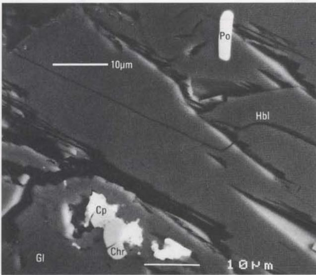
**Figure 12.** Back-scattered electron image of two kinds of sulfides. Sulfides enclosed in hornblende (Hbl) are rounded Ni-rich pyrrhotite (Po), and sulfides in glass (Gl) are irregularly shaped, Cu-rich sulfide (Cp). Fine grains of chromite (Chr) are common. Sample (CH1BB-A) is dome andesite.
