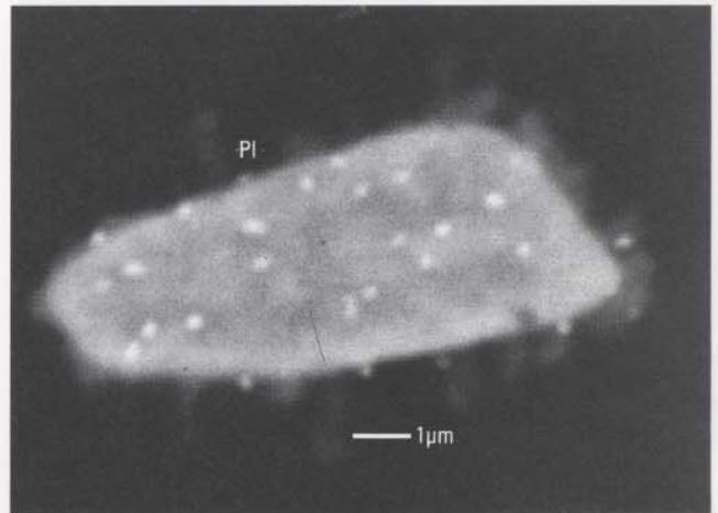
**Figure 14.** Back-scattered electron image showing typical occurrence of Cu-rich sulfides in white pumice. Sulfides in 2-mm-long plagioclase (Pl) phenocryst. The bright portion is the exsolution product of bornite; the dark portion is chalcopyrite (sample PKN 29-2).
