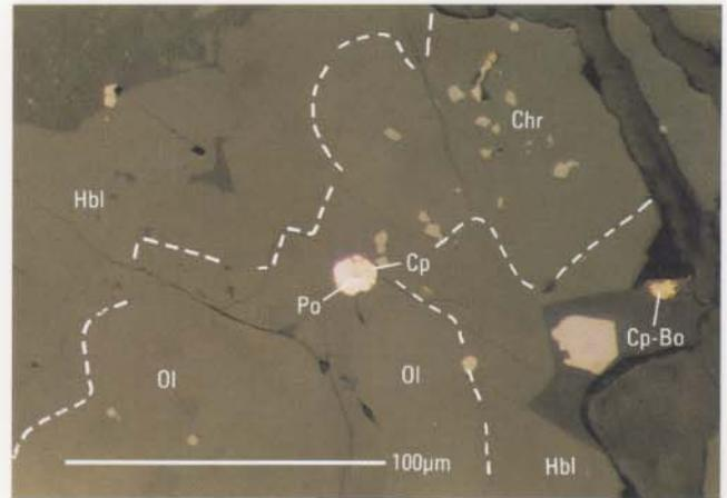
**Figure 13.** Back-scattered electron image of Ni-bearing pyrrhotite (Po) in olivine (Ol) rimmed by hornblende (Hbl) and Cu-rich sulfides (Cp, Bo) in glass. Minute chromite grains (Chr) are visible in olivines. A closeup view of the Po-Cp grain is shown in figure 11. Scale bar is 200 μm.
