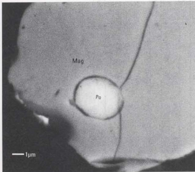
**Figure 4.** Back-scattered electron image of spherical grain of pyrrhotite (Po) in magnetite<sub>ss</sub> (Mag) in dome andesite (sample CN1B-C-X).
