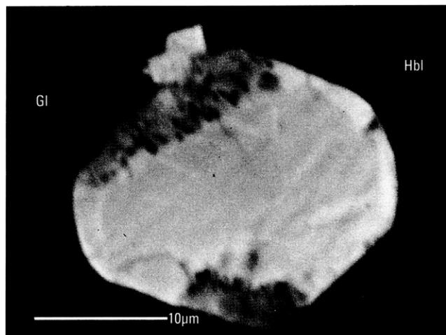
**Figure 17.** Back-scattered electron image of sulfide in white pumice with oxidized rim (sample PP1-A-A). Gl, glass; Hbl, hornblende.
