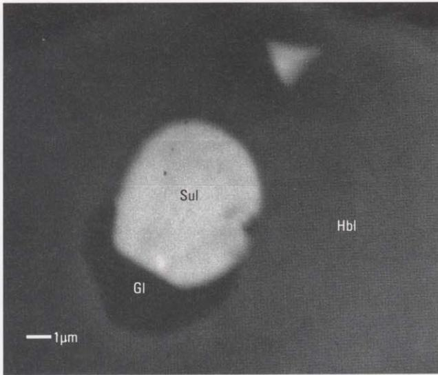
**Figure 7.** Back-scattered electron image of sulfide inclusions (Sul) in hornblende (Hbl) in white pumice (sample PP1-92526-C). Dark area (Gl) surrounding sulfide contains K, Cl, Al, Si, and Fe, and it is interpreted to be a glass inclusion.
