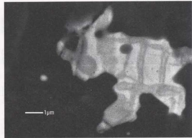
**Figure 6.** Back-scattered electron image of irregularly shaped sulfide grain containing exsolution product of bornite (bright part) in chalcopyrite (darker matrix) in the glass of dome andesite (sample CN1B-D-C).
