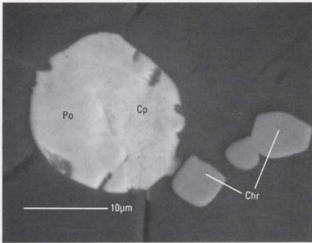
**Figure 11.** Back-scattered electron image of globular Ni-bearing pyrrhotite (Po) in olivine (Ol) rimmed by hornblende (Hbl) and Cu-rich sulfides (Cp) along the cracks of olivine rimmed by hornblende. Chromite (Chr) grains are visible in olivines. A closeup view of the Po-Cp grain is shown in figure 11. Scale bar is 100 μm.
