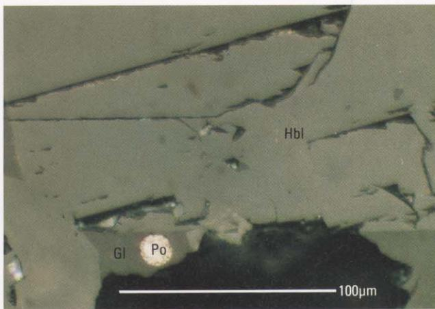
**Figure 8.** Reflected light photomicrograph of spherical grain of pyrrhotite (Po) in basalt glass (Gl) adjacent to hornblende (Hbl).
