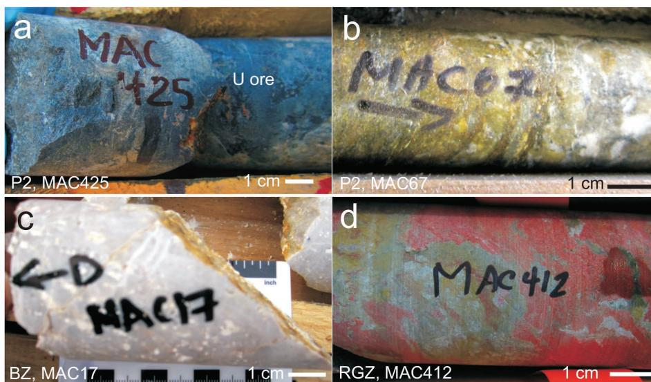
**FIGURE 3.** Photographs of selected drill-core samples; (a) uranium ore of the Zone 2 ore body and P2 fault (MAC425); (b) intensely sudoite-altered pegmatite from the P2 fault (MAC67); (c) quartzite from the Beached Zone along the unconformity (MAC17); and (d) hematitized and chloritized metapelite from the Red-Green Zone (MAC412). Sample locations are shown in Figure 2. (Color online.)
