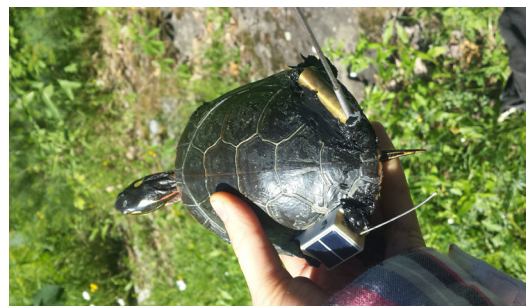
Figure 1. Accelerometer (left) and VHF transmitter (right) attached to the rear carapace margin of a Painted turtle. Photo by Anne-Christine Auge.
