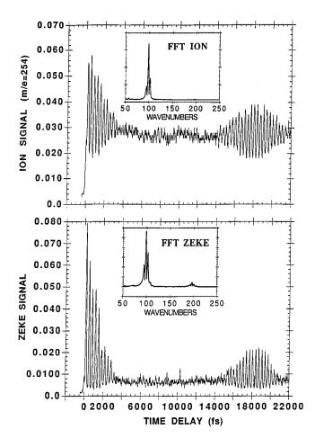
FIG. 2. Long fs pump-probe ion (top) and ZEKE (bottom) scans of the 580 nm  $I_2(B)$  wave-packet dynamics using 345 nm probe (final state,  $v^+=0,1$ ) showing 340 fs modulations. Dephasing and recurrence of the wave packet is seen. The Fourier transform power spectra, inset, show that coherences between vibrational levels v'=14-15, 15–16, 16–17 are involved and that the ion and ZEKE scans contain similar information.
