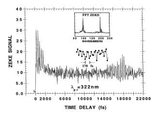
FIG. 3. Long fs pump–probe ZEKE scan of the  $I_2(B)$  wave-packet dynamics using 322 nm probe (final state around  $v^+=20$ ). The complicated pattern contains 170 fs modulations which can be seen on an expanded scale. The Fourier transform power spectrum, inset, shows the significant second harmonic contribution to the signal. Factors affecting the second harmonic are discussed in the text.
