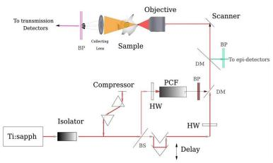
FIG. 1 Schematic of apparatus. A single femtosecond oscillator is used with the Stokes pulse being generated in a PCF. BS = beamsplitter, HW = half waveplate, BP = bandpass, DM = dichroic mirror.
