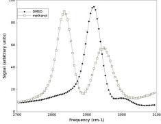
FIG. 2. Doubly-chirped CARS microscopy of methanol, and dimethyl-sulfoxide (DMSO) demonstrating that the doubly chirped technique offers enhancement of spectral resolution.
