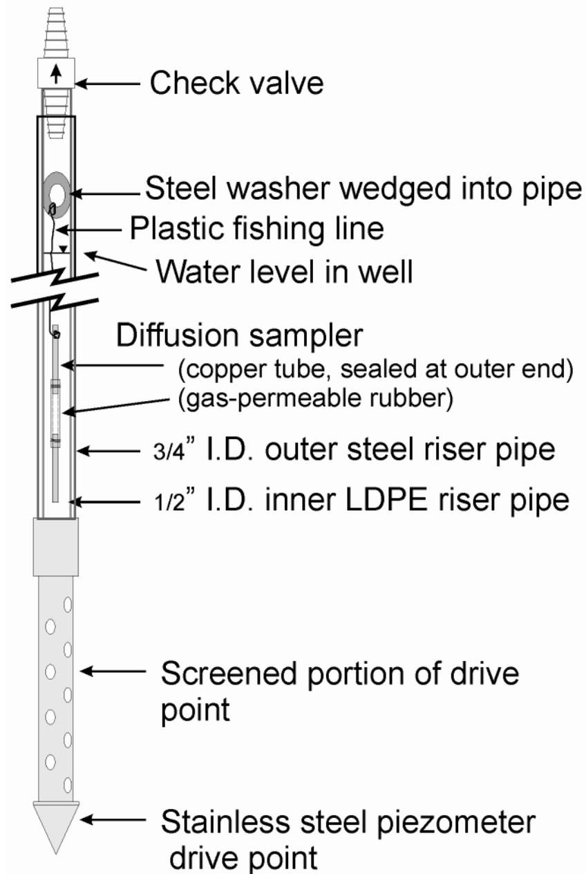
**Figure 19.3.** Design and installation of monitoring well and diffusion sampler (from Hamilton, Hattori and Clark 2005).
