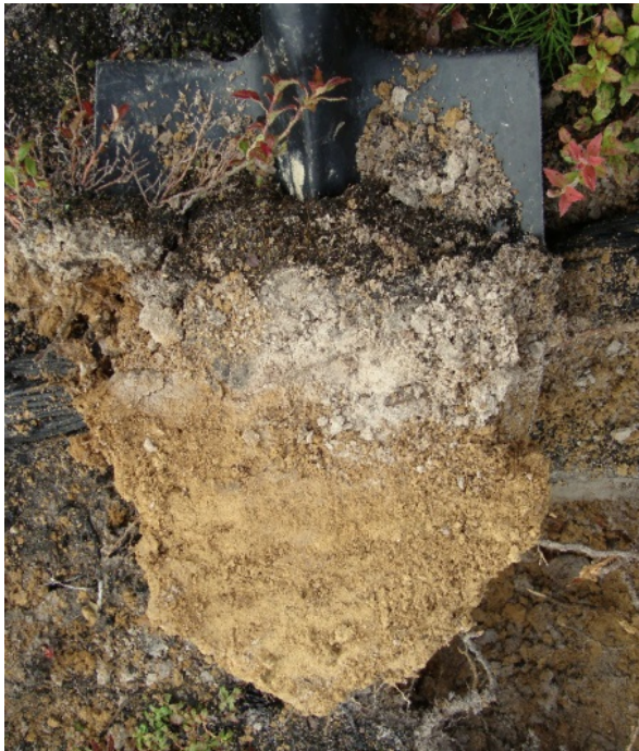
Figure 3. Typical soil profile in the area, showing the black humus, buff-coloured E-horizon and brown B-horizon soil in the Millennium property.
