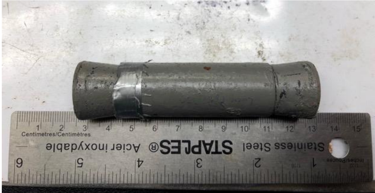
Figure 1-7. Physical models of Yarrow's spiny lizards ( Sceloporus jarrovi ) made of hollow copper piping, painted grey to mirror the reflectance of these lizards. Ruler included for scale in centimetres.
