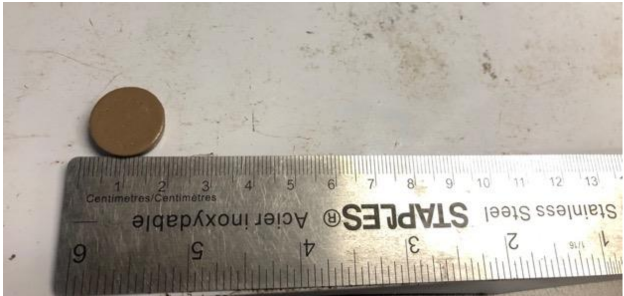
Figure 2-5. Physical models of ornate tree lizards ( Urosaurus ornatus ) made by painting a Thermochron iButton DIS1921G-F5 temperature logger brown to mirror the reflectance of these lizards. Models were placed throughout ten sites in the Chiricahua Mountains, Arizona, USA. Ruler included for scale in centimetres.
