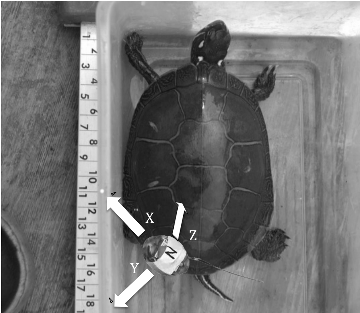
Figure 3-1 – Placement of accelerometer device on left side of a tagged painted along with a radio transmitter. Arrows show direction of x, y and z-axis.
