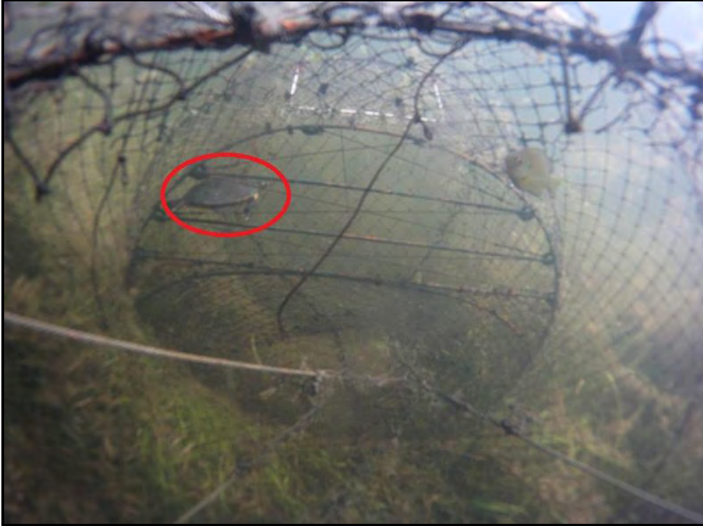
Figure 8: An adult painted turtle passing through the selective “grid” of the prototype escape device in situ in Lake Opinicon, Ontario, Canada. Bars spaced 8 cm apart and diagonally stretched tarred twine serve as a selective barrier.
