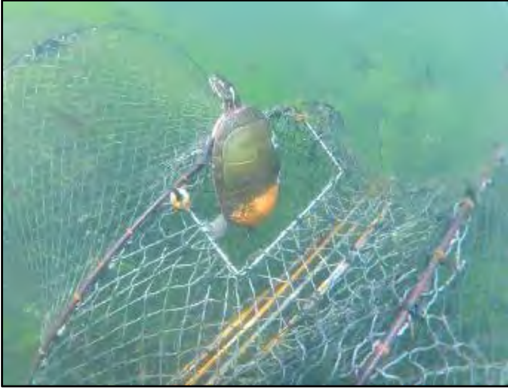
Figure 9: An adult painted turtle passing through the 22.5 X 10 cm escape hatch of the prototype grid escape device during controlled preliminary trials in Lake Opinicon, Ontario, Canada.
