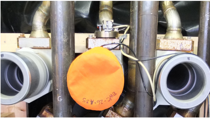
(Left) AECL's Composite Angle Profiling Tool (CAPT) tool mounted on a full-size mock up of a CANDU reactor's feeder piping. The tight spaces and angled surfaces provide ample technical and physical challenges.
