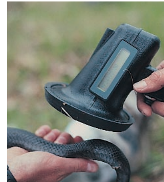
The reader passes over an embedded microchip to get a positive I.D.
